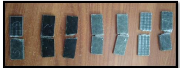
Figure 42 impact strength specimens of all materials
