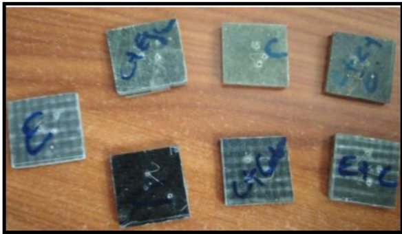
Figure 43 hardness testing specimens
